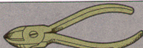
Pliers, NSN 5110-00-239-8253 Diagonal Cutting 6-in long
